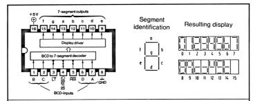
**Description:**This device converts BCD input data into control signals for 7-segment displays.
