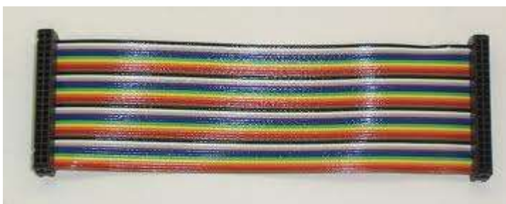
Figure 2. 20 The ribbon cable for connecting computer peripherals
