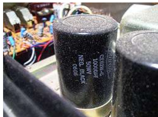
Figure 2. 41 A reservoir capacitor in an amplifier
